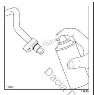
☐ Clean the surface and the seal of the pipe using EN-GINE CLEANER (see Vehicle: Parts and consumables for the repair) (04B, Consumables -Products).
