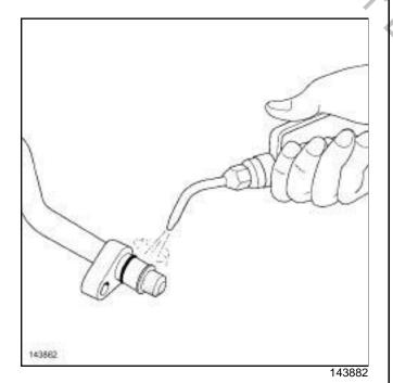
☐ Use a **compressed air gun** to blow the surface and the seal of the connecting pipe.
