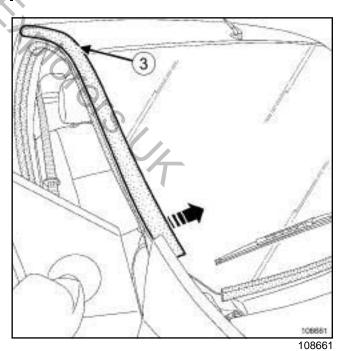
☐ Remove the frame seal (3).
