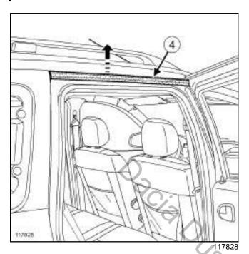
☐ Remove the frame seal (4).
