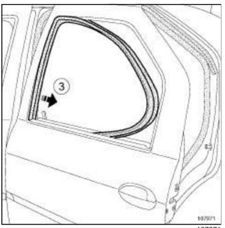
☐ Remove the rear side door window run channel at (2) and (3).
